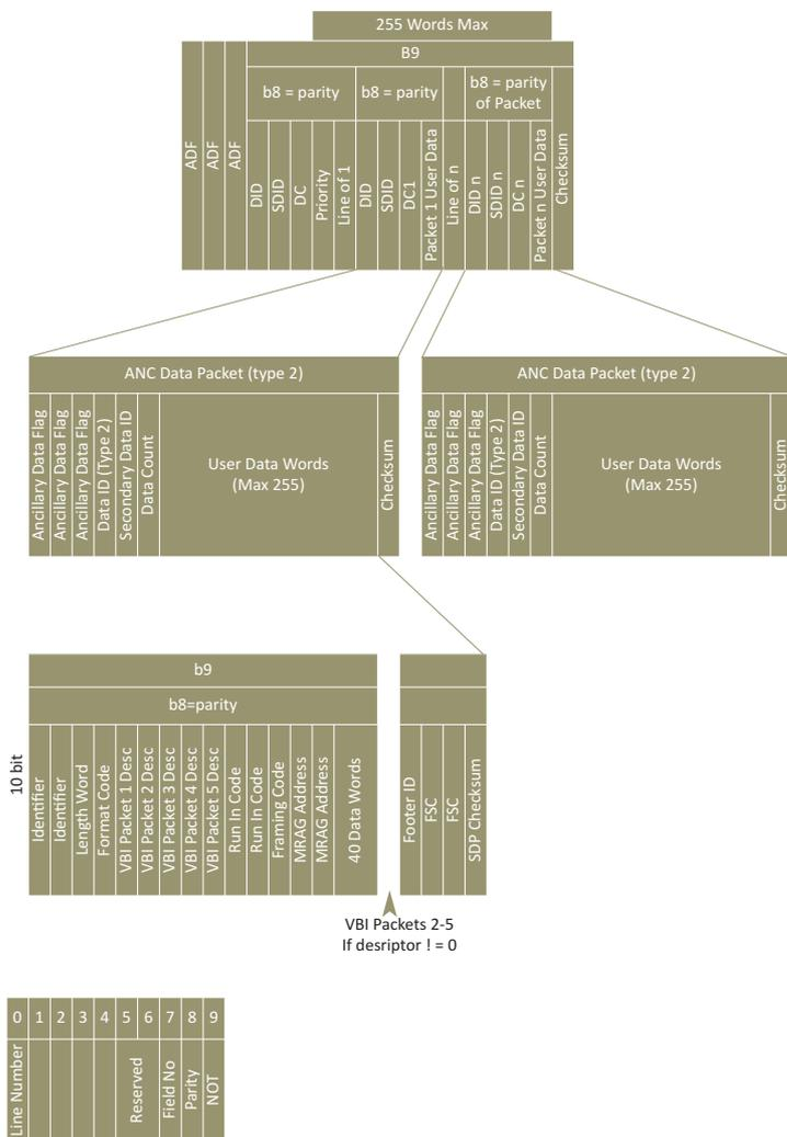
**Fig 2: showing the format of Type 2 Ancillary Data in a VANC multipacket. Type 1 ancillary data has similar format with the Secondary Identifier (SDID) replaced by a Data Block Number (DBN) Type 1 is more commonly used for Audio data**
